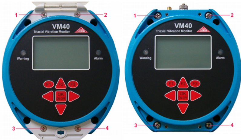
Figure 33: Removing the plastic cover and opening the casing
