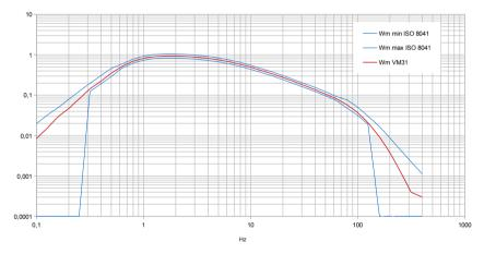
Figure 1: Frequency response of the weighting filter Wm
