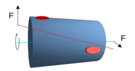
Dynamic unbalance: Mass axis not parallel and not intersecting rotational axis at center of gravity
