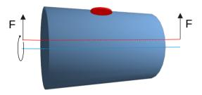
Static unbalance: Mass axis parallel to rotation axis
