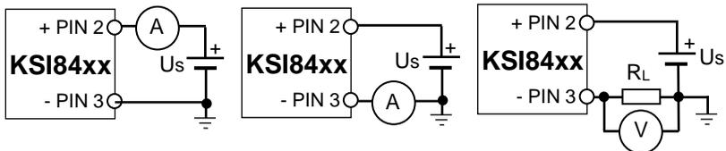
The sensor current can be measured either directly by a current meter connected in series or indirectly by measuring the voltage drop across the load resistance  $R_L$  between PIN 3 and the negative terminal.
