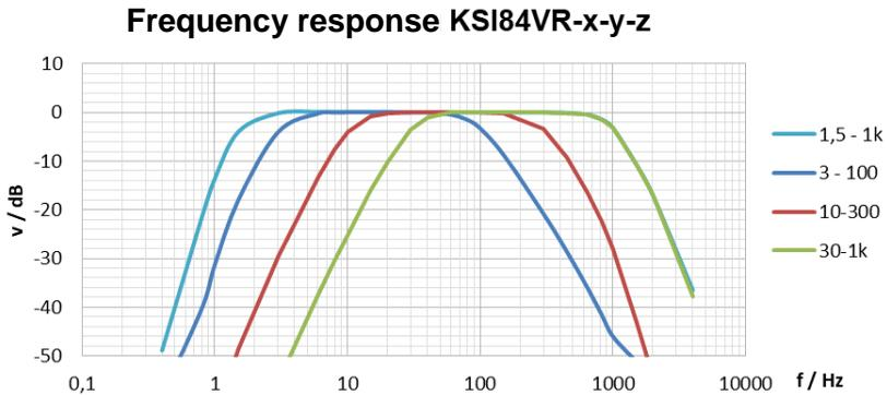
The HP filter of the **displacement** sensor types has a stopband attenuation of -60 dB/decade. The upper cut-off frequency is 300 Hz. It results from the significant decrease of the [dynamic range](#) with increasing frequency. At 300 Hz the maximum current amplitude is only 1 % of the [measuring range](#).
