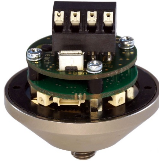
Figure 1: Open VS11 with terminals for power supply / relay output and USB socket
