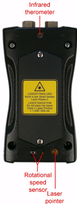
Figure 34: Rotation speed and temperature sensor, laser pointer
