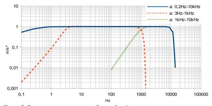
Figure 3: Frequency response curves for acceleration
