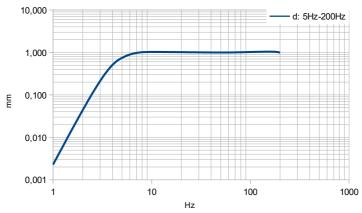
Figure 6: Frequency response curves for displacement
