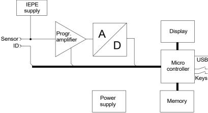
Figure 2: Block Diagram
