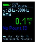
Figure 18: Measurement display
