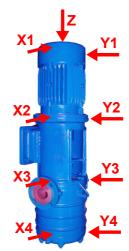
Figure 16: Measuring points on machines with vertical rotors
