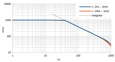
Figure 5: Amplitude range for velocity (RMS)
