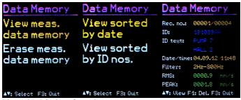
Figure 25: Display of saved measurements
