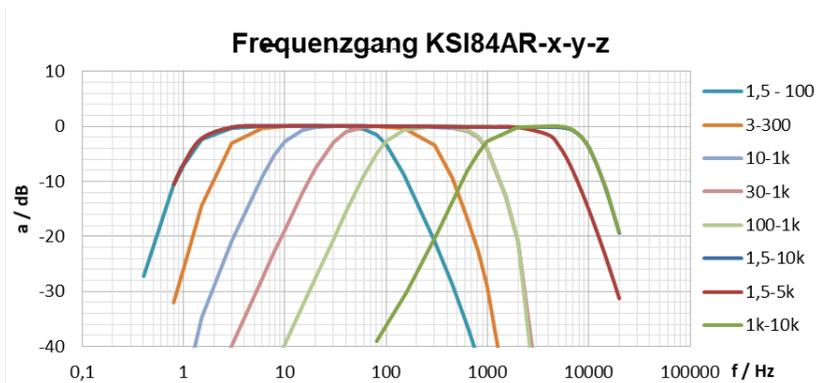
The HP filter of the **velocity** sensor types has a stopband attenuation of -50 dB/decade, the LP filter has a stopband attenuation of -40 dB/decade.
