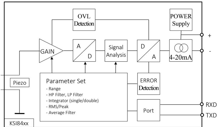
The sensors of the KSI84xx family are piezoelectric vibration sensors.
