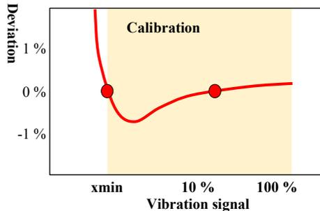
At vibration amplitudes **greater** than the maximum  $x_{\text{max}}$ , the sensor current no longer increases. It remains constant at **22 mA**<sup>1)</sup>. A sensor with a larger measuring range must be selected.
