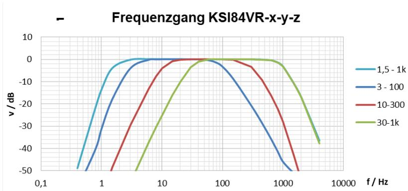
The HP filter of the **displacement** sensor types has a stopband attenuation of -60 dB/decade. The upper cut-off frequency is 300 Hz. It results from the significant decrease of the [dynamic range](#) with increasing frequency. At 300 Hz the maximum current amplitude is only 1 % of the [measuring range](#).
