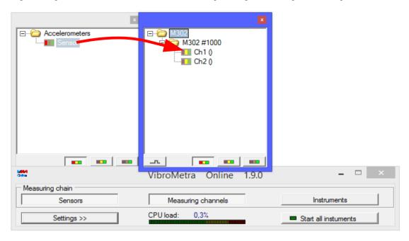
8. Click "Instruments" to see the list of available software licenses. The licenses are stored inside your M302/M312 device. Installed licenses are marked yellow/green. An instrument is opened by a double click.
