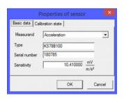
7. Click "Measuring channels". You will see type and serial number of the connected USB device(s). Drag and drop a sensor onto the correct M302/M312 input using the mouse pointer with pressed left button.
