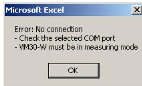
Figure 11: Transmission error
