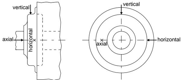
Figure 3: Measuring points on end shield bearings
