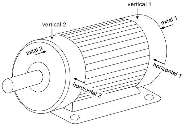
Figure 4: Measuring points on electric motors
