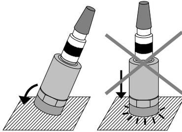
Figure 5: Attaching the magnetic clamp
