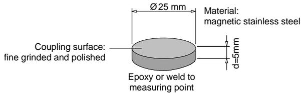
Figure 6: Preparing the coupling point
