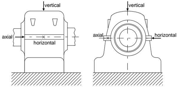
Figure 2: Measuring points on pillow block bearings
